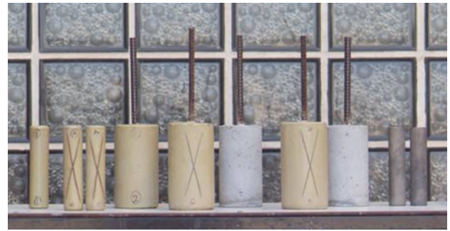
Fig. 2 Photograph of the test samples after exposure to atmospheric test
