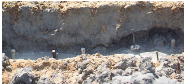
Fig. 6 Photograph of the test samples in the trench after burying in the sabkha soil
