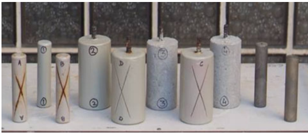
Fig. 3 Photograph of the test samples after immersion in 5% NaCl
