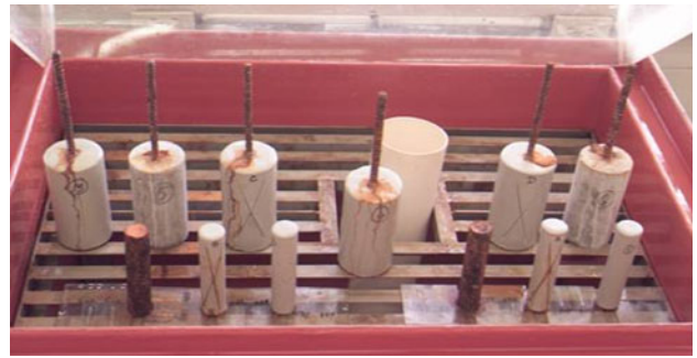
Fig. 5 Photograph of the test samples after salt-spray test
