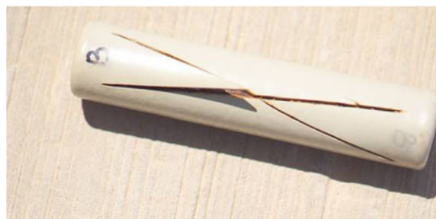
Fig. 16 Photograph showing detachment of the coating from the steel substrate
